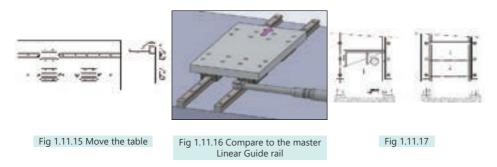
% Sample Installation of the Linear Guide without a Reference Section for the Master Linear Guide Rail.
