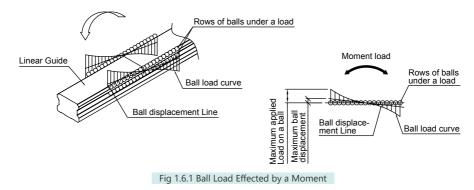
An equivalent-load equation applicable when a moment acts on a Linear Guides is shown below.
