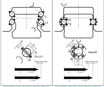
Fig 1.1.1 Four-Row Equal Load Ratting Design
