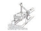
Fig 1.11.19 Use a Temporary Reference Surface
