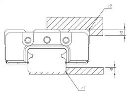
Table 3.1.5 Height of shoulder and chamfer
