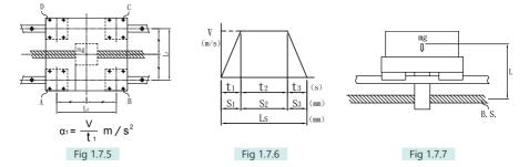
(2) Load Applied to the Linear Guide Block
