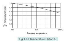
When used at ambient temperatures higher than 80°C, the seals, end caps, and ball cages used must be changed to those with hightemperature specifications.
