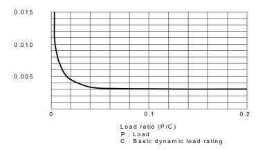
Linear guides enable load movement using rolling elements like balls or rollers, resulting in friction that is 1/40th of the one found in traditional sliding systems. The causes of friction include the viscous resistance of lubricants, preload friction resistance, and friction generated by the applied force. The diagram above illustrates the coefficient of friction when the linear guide is subjected to force.
