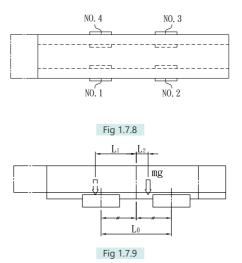
(2) Load applied to the Linear Guide block
