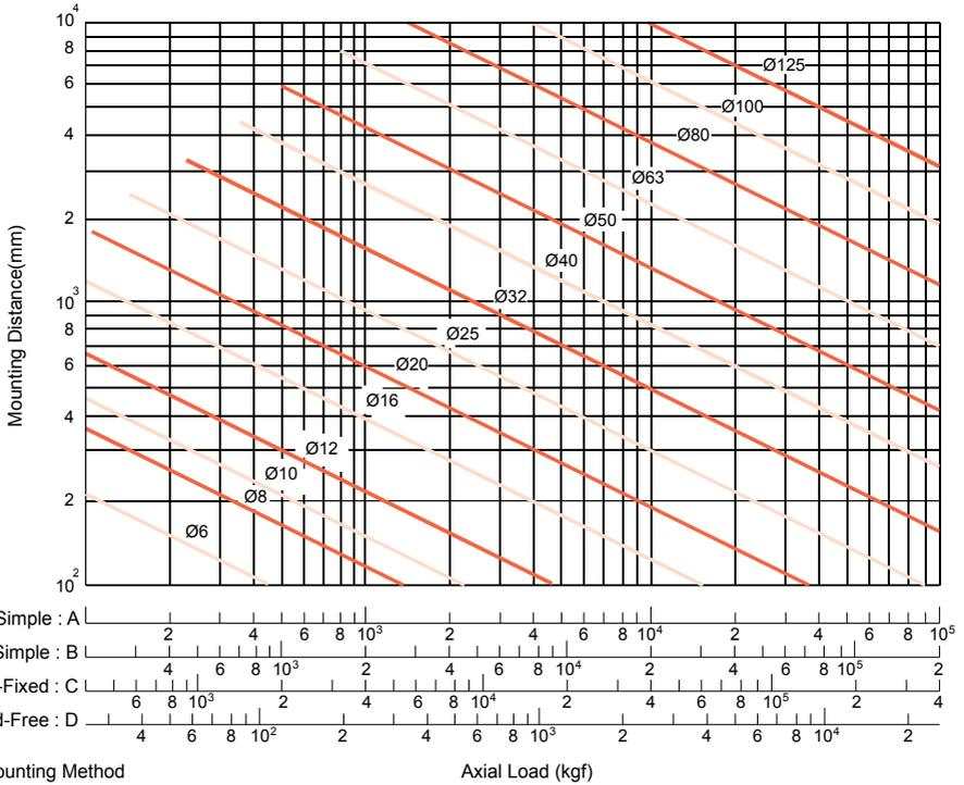
Fig 1.4.16 Buckling Load vs. Nominal Diameter and Length
