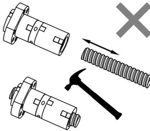
Fig 1.10.1 Error installation
