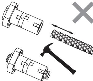
Fig 1.10.1 Error installation
