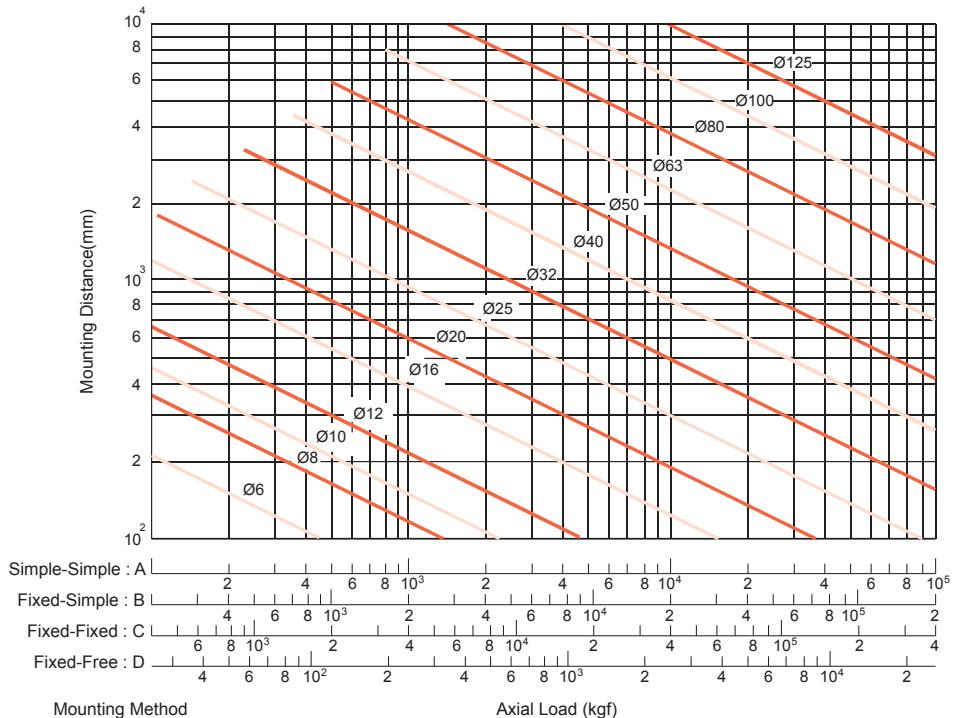
Fig 1.4.16 Buckling Load vs. Nominal Diameter and Length
