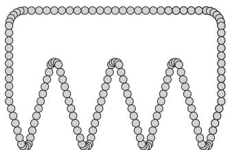
Fig 1.1.3 External Ball Circulation Nuts
